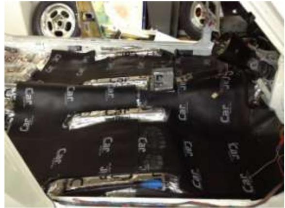
The floor was covered in acoustic deadening sheeting including underneath the dash panels and over the gear selector housing. All unnecessary holes in the sills etc. were also covered to prevent water / dust ingress. I then used a car acoustic underlay and finally a new carpet set.
