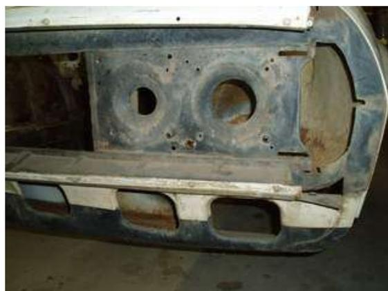
Front of car shows surface rust in panel under bumper bar and evidence of work carried out by dealer to get front indicator lights and associated panels to fit properly.
