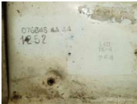
As can be seen in this photo (without compliance plate), the compliance number is P76 076 B4S4 A44 1252 with a build date of 7/73. The engine number is 4404/1259 and as you can determine came without air conditioning.
