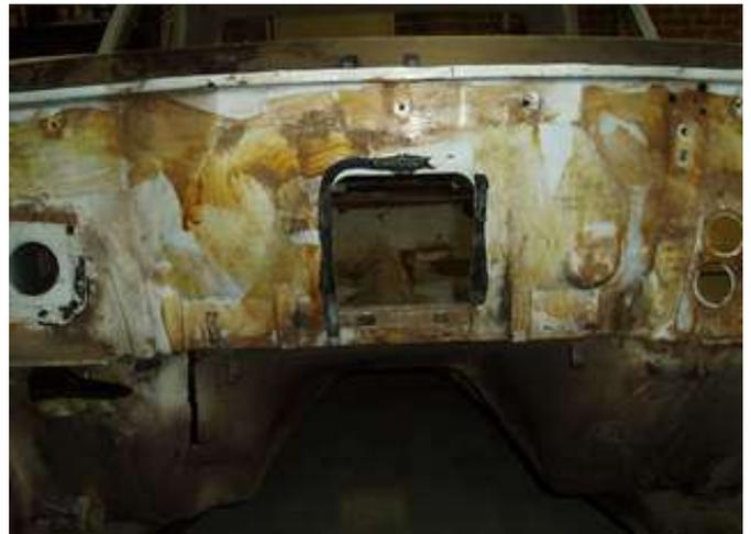
Original positioning of sound deadener under the window wipers. Firewall showing haphazard placement of yellow glue and luckily no signs of rust.
